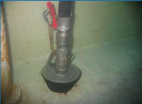
Shaped plug for deeper tanks
