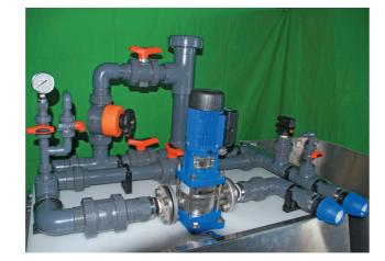
There is a safety mechanism for 'no flow' situations and a diaphragm valve for fine tuning the chlorine infusion module.
