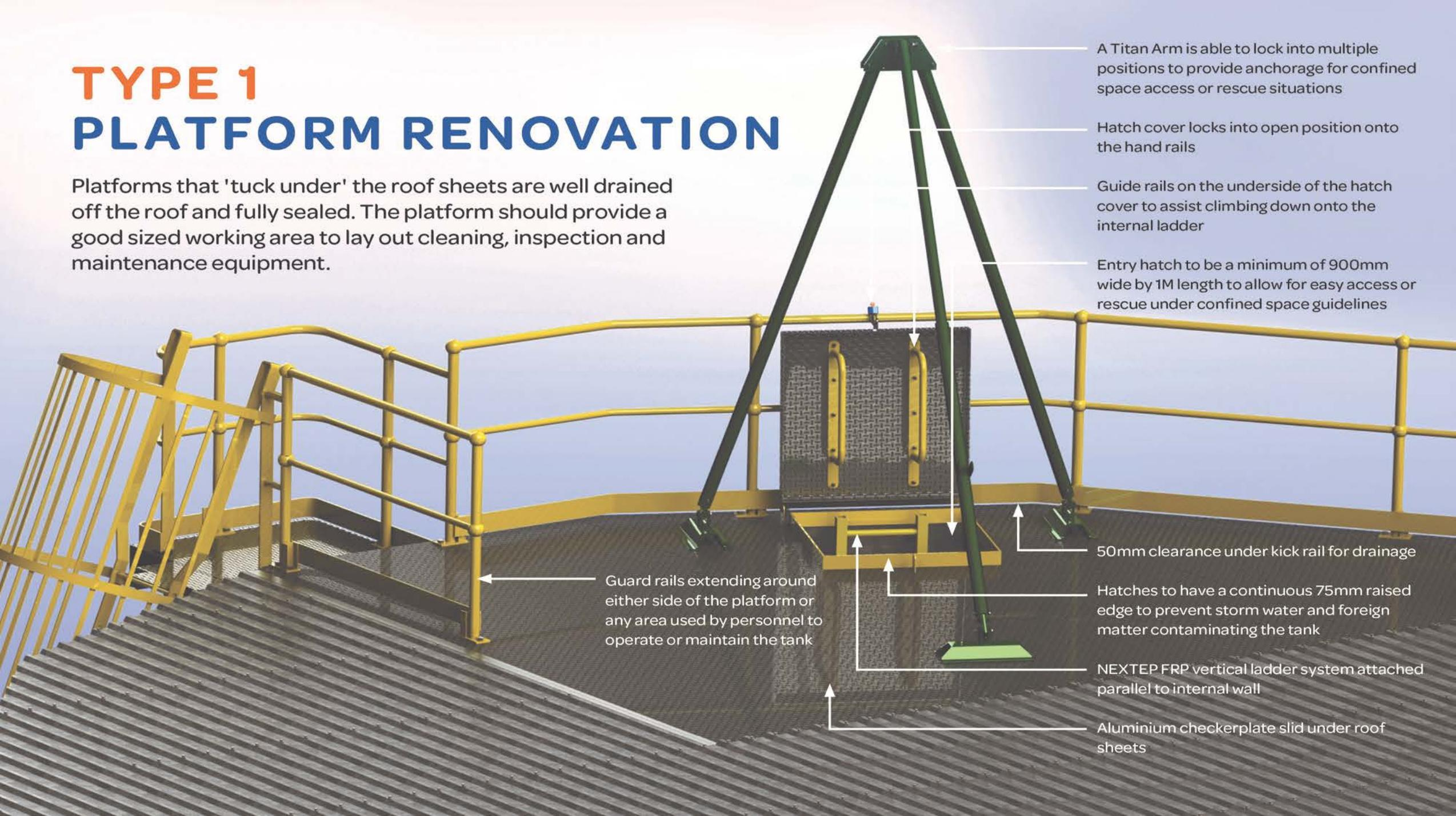
A Titan Arm is able to lock into multiple positions to provide anchorage for confined space access or rescue situations
