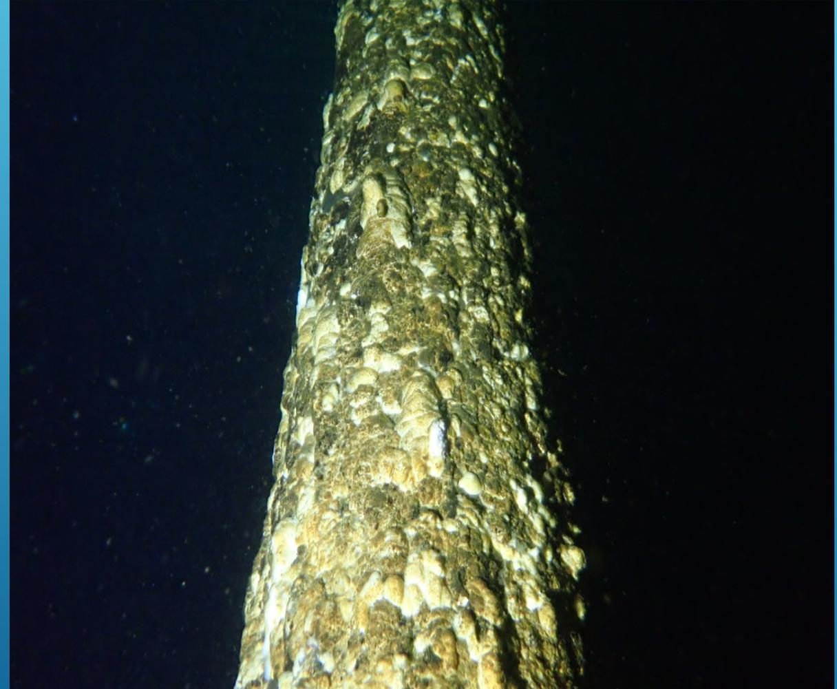
Aluminum ladders corrode quickly in some waters, depending on pH levels. The SS bolts also contribute to the aluminum deteriorating.
